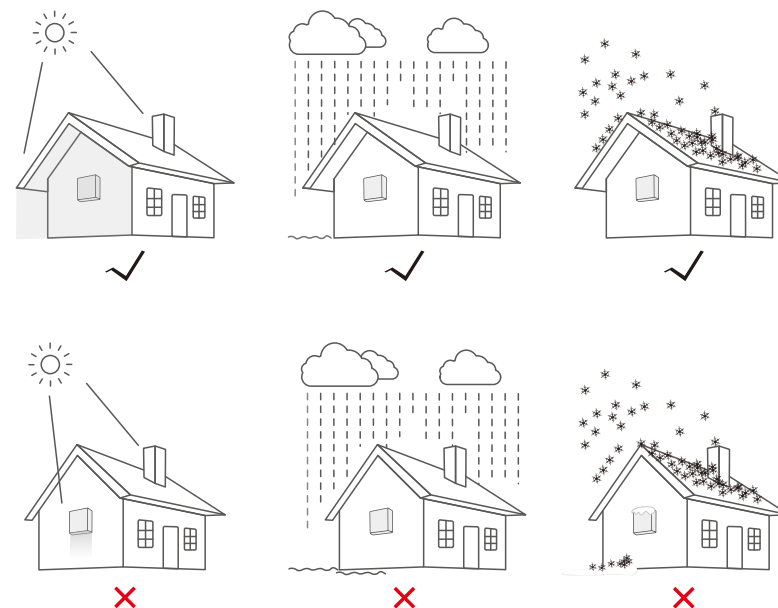
▲ Figure 4.1 Recommended Installation locations
